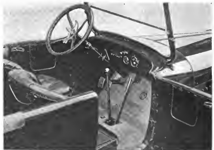
Driver's compartment of new Lexington, showing divided front seats, ample leg-room and control members
